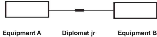
The *Diplomat jr* models are all designed to connect two pieces of equipment using serial RS232 data streams operating at different data rates and character formats.
